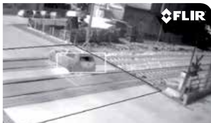
Level crossing obstacle detection
