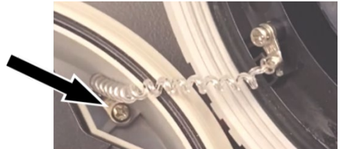
FIGURE 3-1: ATTACH ANTI-DROP CABLE TO CAMERA
