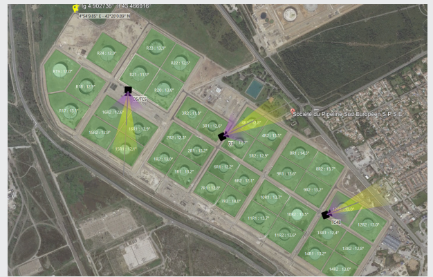
Only by using three camera systems, each of the forty tanks on the site are automatically scanned every three minutes during 50 seconds.
