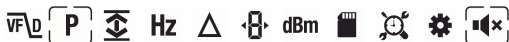
Figure 5.3 Mode icons (AC voltage measurements): Peak mode and Silent mode are enabled
