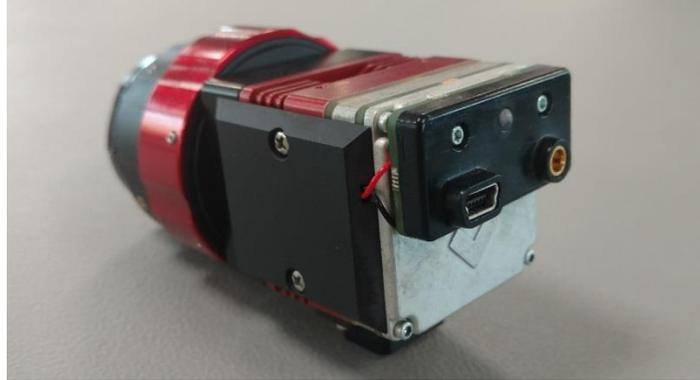
**Figure 8** Tau SWIR with VPC module and cover plate.
