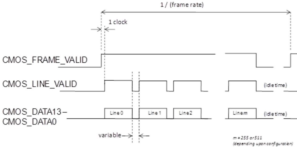
**Figure 10 Frame Timing CMOS Protocol**
