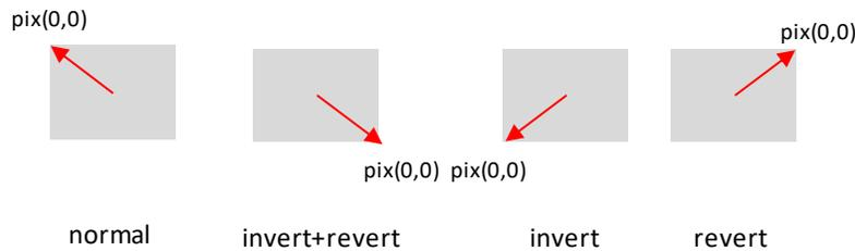
**Figure 18 Illustration of Image Orientation Modes**
