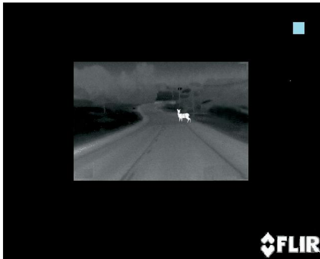
Figure 1. Example image of Half Zoom. This can be achieved by clicking ‘Unzoom’ in the GUI. No zoom indicator, and FFC icon in upper right. Sensor resolution = Display resolution. (FLIR logo present in some versions.)
