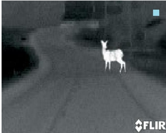
Figure 3. Example image of 2X Zoom. This can be achieved by clicking 'Zoom 4X' in the GUI. No zoom indicator, and FFC icon in upper right. Image shown with Zoom level indicator off. One pixel on sensor = 4x4 on display. (FLIR logo present in some versions.)
