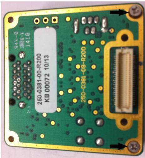
Figure 11: Philips screws to remove
