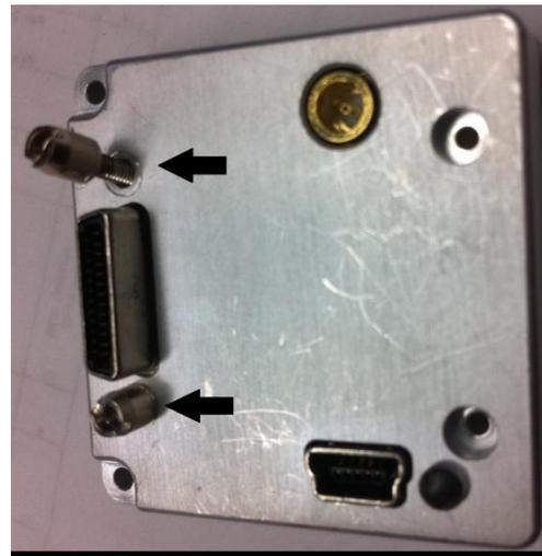
Figure 12: Jack Screws to remove
