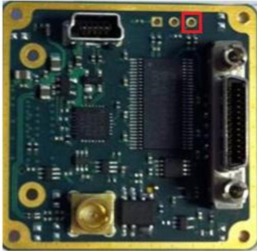
**Figure 19: Ext Sync Header Connection**
