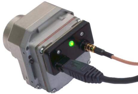
Figure 3: VPC Physical Connections
