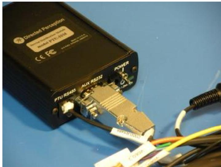
2. Now plug the RS232 connector at the end of the breakout cable into the "AUX RS232" port of the ISM module. Then plug the RS485 connector from the breakout cable into the ISM module's "PTU RS485" connector.
