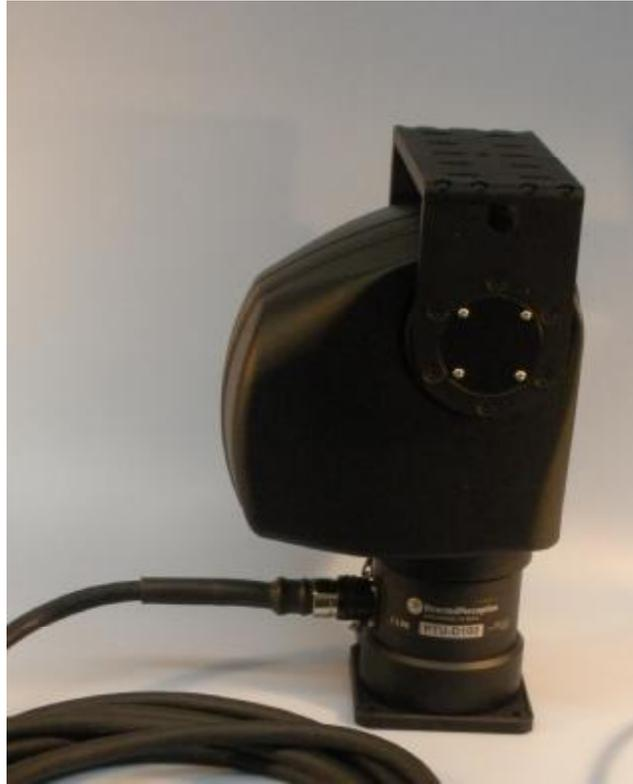
1. The first thing you need to do is plug in the 25' breakout cable into the D100.
