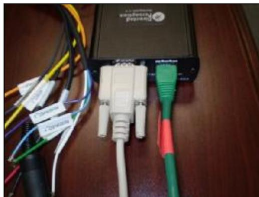
4. You have now completed all connections to the D100; the only remaining items are to connect the ISM to the network, and to connect the RS232 communication between your PC and the ISM module. Do this by using the included cross over Ethernet cable to directly connect the Ethernet port on the ISM module to the Ethernet port on your computer. Finally, connect an RS232 9 port serial cable to the "Control RS232" serial port on the ISM and to an open serial port on your computer.
